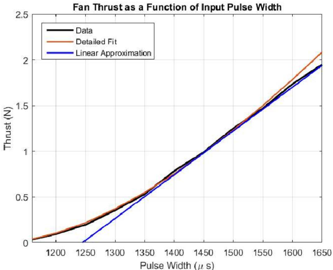
This looks pretty good! We can adjust the offset if we want to minimize error, but we might as well just leave it and see how it works. The next thing is to make a linearized dynamical model and see if its steady state response matches this.
