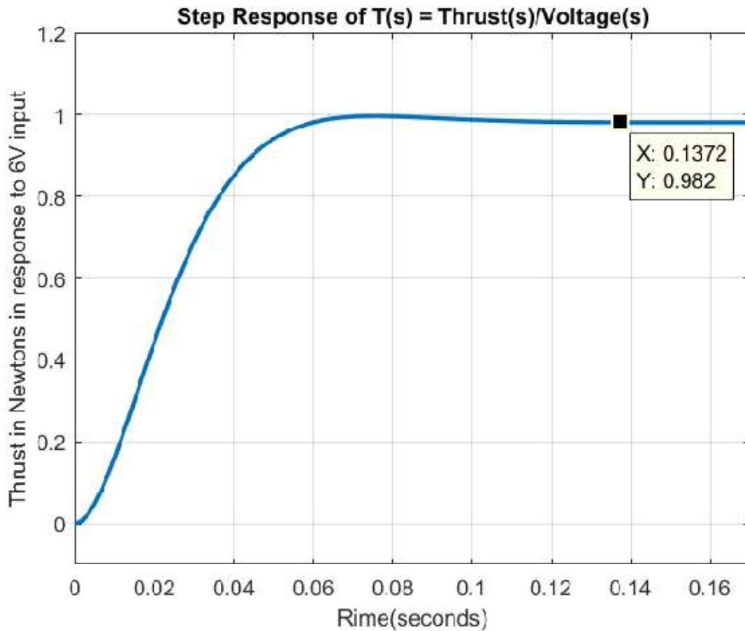
Another important thing to remember is that I totally guessed the coil inductance and the moment of inertia of the rotor/prop. Well, not totally guessed: I judged the size, core material and number of turns based on pictures of the motor, and I assumed that the rotor weighted 10 grams and that its moment of inertia can be approximated by a ring of mass at a distance around where the magnets are. Measuring these things could help.
