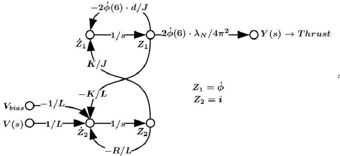
So, K is known, R was calculated, d was calculated, n(6) is known... but J and L are unmeasured. These parameters determine the speed of the system. I tried to figure them out by looking at pictures of the motor and propellor, and finding out how much they weigh, and guessing things.
