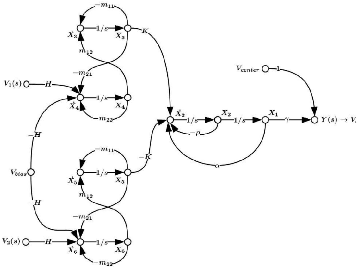
I also added another input  $V_{center}$ , which is 2.5V with our current setup.
